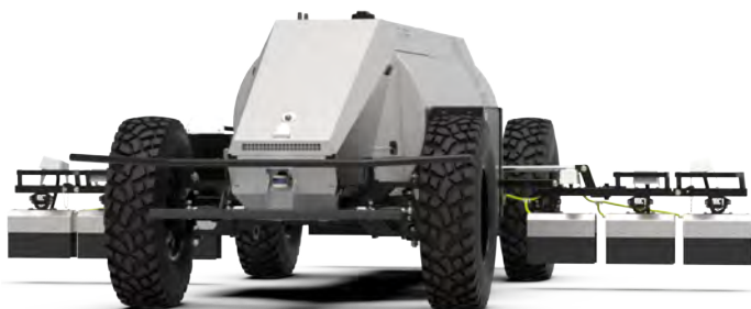
Photo via GUSS | The classic GUSS has been kicked up a notch, now running on electric power as an autonomous sprayer platform.
