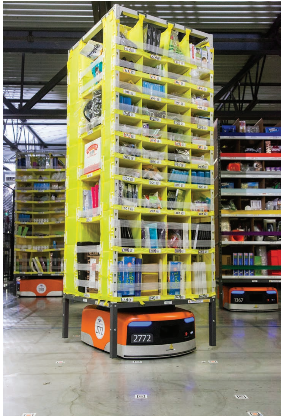
PHOTO VIA AMAZON | Amazon's "Kiva" robots are part of the suite of automated systems used in e-commerce fulfillment centers.
